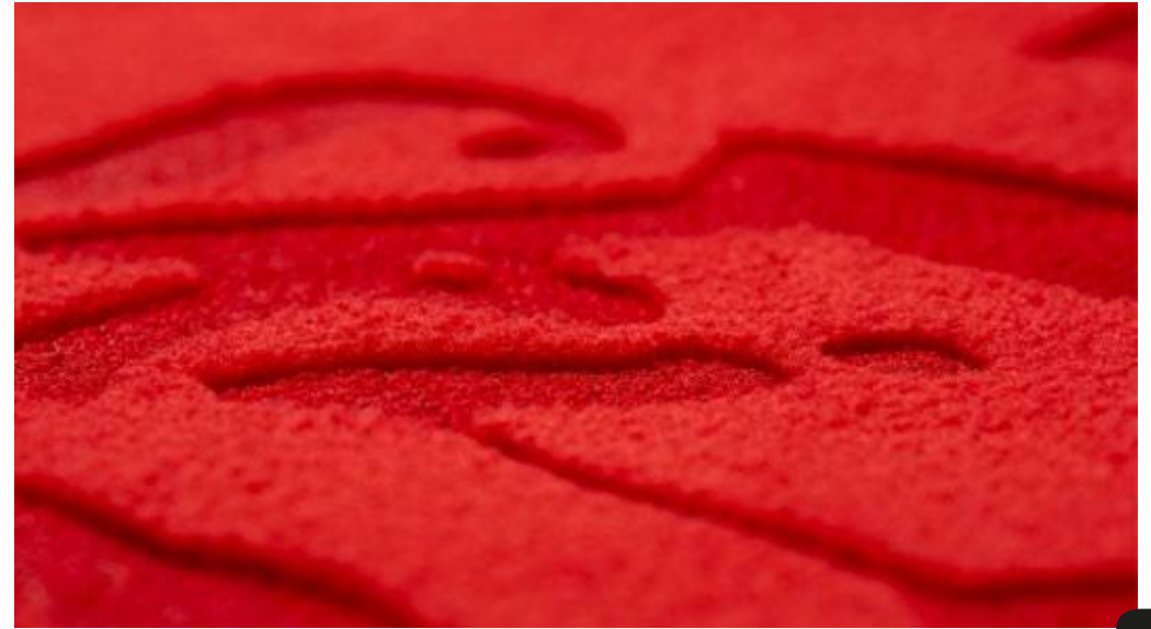
»»»» Gravure laser. Laser engraving.
